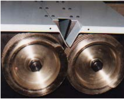
View with safety guard removed showing the sharpening wheels
